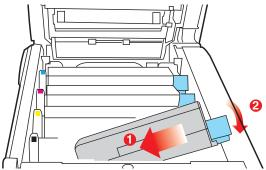
**10.** Pressing gently down on the cartridge to ensure that it is firmly seated, push the coloured lever (1) towards the rear of the printer. This will lock the cartridge into place and release toner into the image drum unit.
